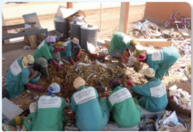
Women's association sorting and recovering waste plastics in Ouagadougou (sorting by colour and material, manual cleaning, mechanical grinding). The ground material is sold to casting plants that manufacture plastic products.
